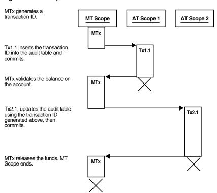
Figure 2-6 Example: Bank Withdrawal—Sufficient Funds
