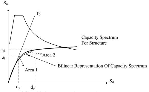
Figure 4. Bilinear representation of capacity spectrum
