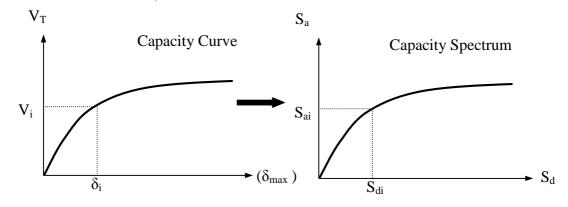
Figure 2. Conversion of capacity curve to capacity spectrum
