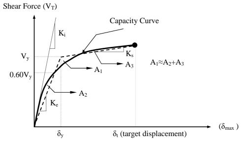
Figure 7. Idealization of capacity curve
