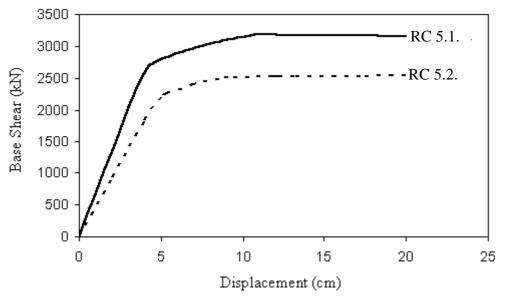
Figure 10. Capacity curves of the five-storey reinforced concrete 3D frame system structures
