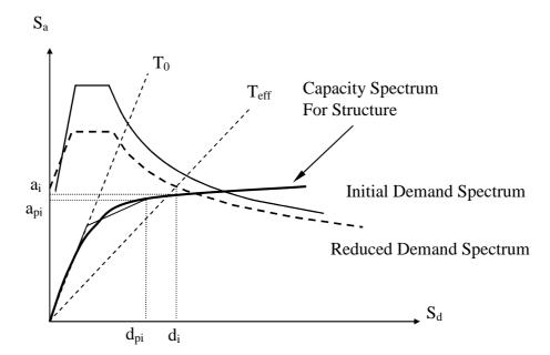
Figure 5. Determination of estimated maximum displacement using direct iteration
