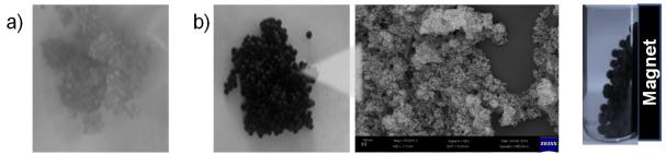
**Figure 2**. Photograph of Cefazolin encapsulating a) alginate macrobeads (2%) and superparamagnetic nanoparticle (SPION) embedded alginate macrobeads. FE-SEM image of SPION clustered on alginate bead surface and image demonstrating the magnetic properties of the resulting macrobeads
