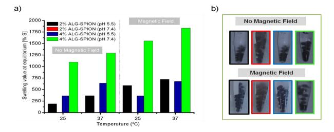
**Figure 4.** a) Effect of pH, temperature and magnetic field on the swelling value of the hydrogel at equilibrium depending on the initial alginate concentration of the ALG- SPION macrobeads and b) images depicting the effect of swelling after 24 hours at 37  $^{\circ}$ C (Frame colour of each image corresponds to legend color of the samples depicted in the graph. Experiments were carried out with 0.2 g/1 mL hydrogel
