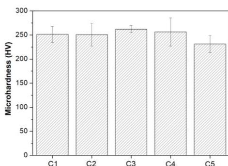
**Figure 5.** The hardness of the coatings prepared with different concentrations of Nickel chloride in the bath
