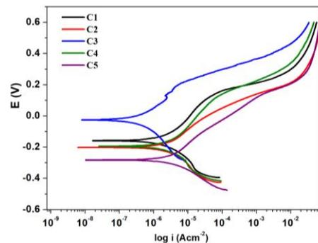
Figure 4. Potentiodynamic polarization curves of the investigated coatings.
