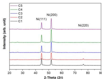
**Figure 1.** X-ray diffraction patterns of Ni coatings produced at different concentrations of nickel chloride.
