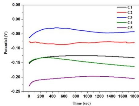
Figure 3. Evolution of open circuit potential ( $E_{oc}$ ) vs. time.
