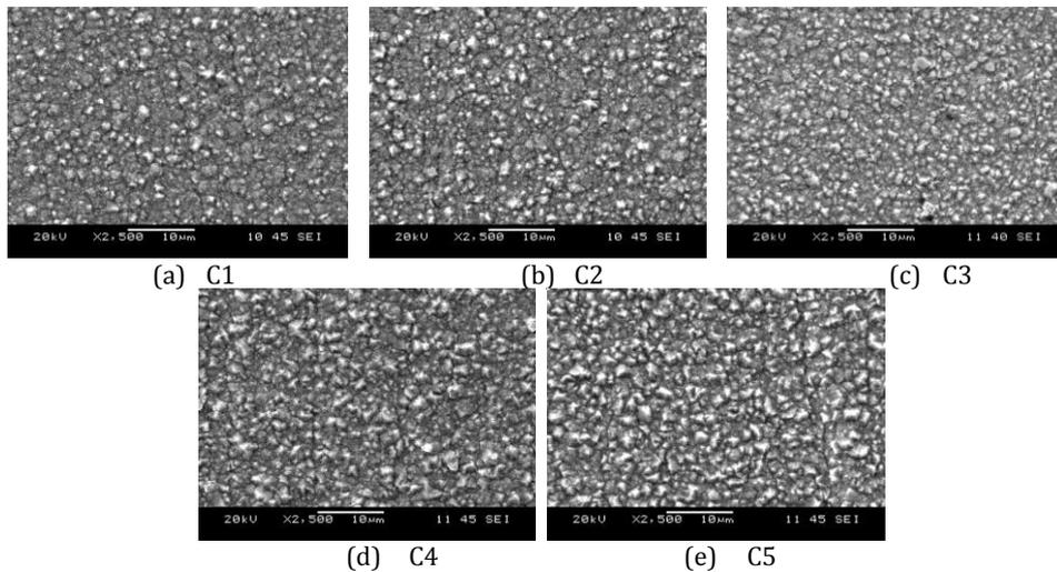
**Figure 2.** Surface morphology of nickel coatings with different concentrations of Nickel chloride in the bath.
