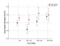
**Figure 4.** Change in the Izod impact strength of PS samples with filler reinforcement before and after gamma irradiation.
