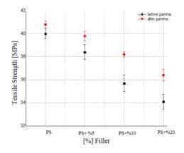
**Figure 2.** Change in the tensile strength of acorn powder reinforced PS samples before and after gamma irradiation.
