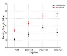
**Figure 6.** Change in the three-point bending strength of filler-reinforced POM samples before and after gamma irradiation.
