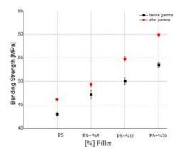
**Figure 3.** Change in the three-point bending strength of PS samples with filler reinforcement before and after gamma irradiation.
