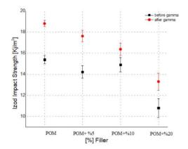
**Figure 7.** Change in the Izod impact strength of filler-reinforced POM before and after gamma irradiation.
