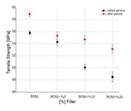
**Figure 5**. Change in the tensile strength of fillerreinforced POM samples before and after gamma irradiation.
