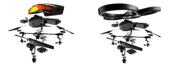
Figure 1. AR Drone quadcopter disassembled view
