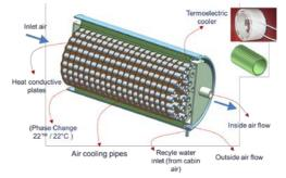
Figure 9. Newly developed cold storage system
