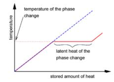
Figure 8. Storing heat at steady temperature [10]
