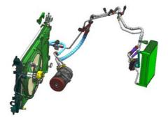
Figure 2. Current air conditioning cooling group
