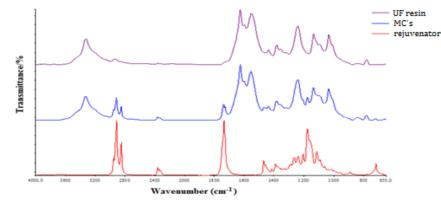
Figure 4. FTIR spectrogram of microcapsule and rejuvenator.
