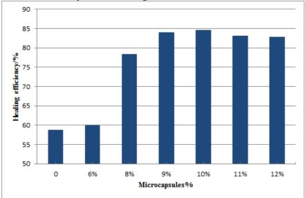
Figure 6. The healing performance of asphalt with microcapsules under low temperature conditions (5°C).
