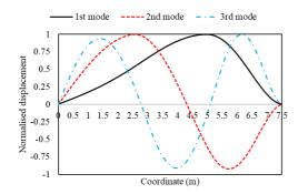
**Figure 4.** First three mode shapes of segmented Timoshenko beam on Pasternak foundation with S-F boundary conditions ( $K_W = 50$ ,  $K_S = 4$ )
