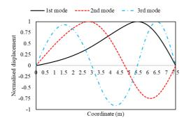
**Figure 3.** First three mode shapes of segmented Timoshenko beam on Pasternak foundation with S-S boundary conditions ( $K_W = 50$ ,  $K_S = 4$ )
