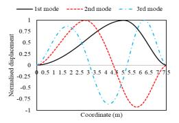
**Figure 6.** First three mode shapes of segmented Timoshenko beam on Pasternak foundation with F-F boundary conditions ( $K_W = 50$ ,  $K_S = 4$ )
