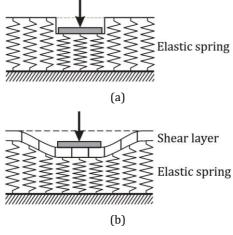
Figure 1. Displacement of a) Winkler b) Pasternak foundation models [1]
