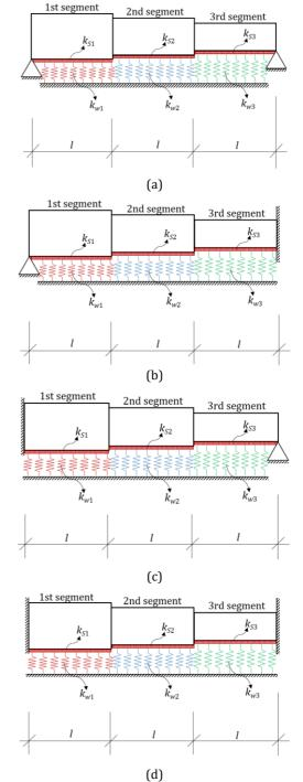
**Figure 2.** Mathematical model of segmented Timoshenko beam on Pasternak foundation for a) S-S b) S-F c) F-S d) F-F boundary conditions
