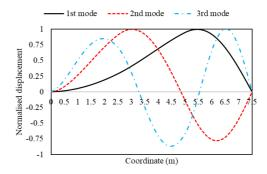
**Figure 5.** First three mode shapes of segmented Timoshenko beam on Pasternak foundation with F-S boundary conditions ( $K_W = 50$ ,  $K_S = 4$ )
