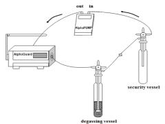
**Figure 4.** Schematic view of the AquaKIT measuring set-up in water
