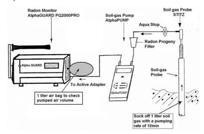
Figure 2. Schematic set-up of AlphaGUARD radon-thoron monitoring in the soil gas.
