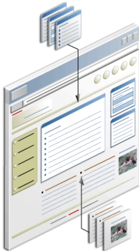
Figure 16-1 Portal Content Is Comprised of Portlets and Items
